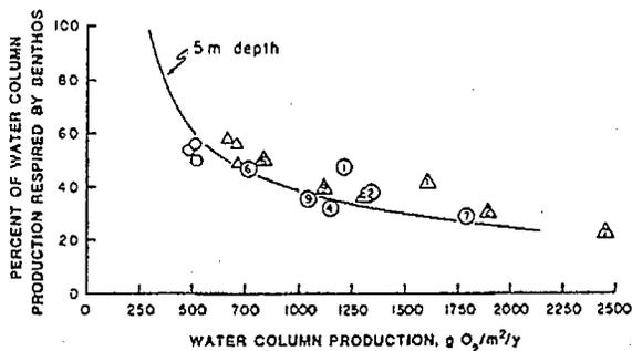
Fig. 10. Benthic respiration as percent of water column production respired by benthos versus water column production. (C) Period Jun 1981 to Jun 1982; ( $\Delta$ ) Jun 1982 to Jun 1983. Numbers refer to individual mesocosm treatments (see Table 1); unnumbered symbols are controls. The line is for a 5 m deep water column (from Hargrave 1973)
